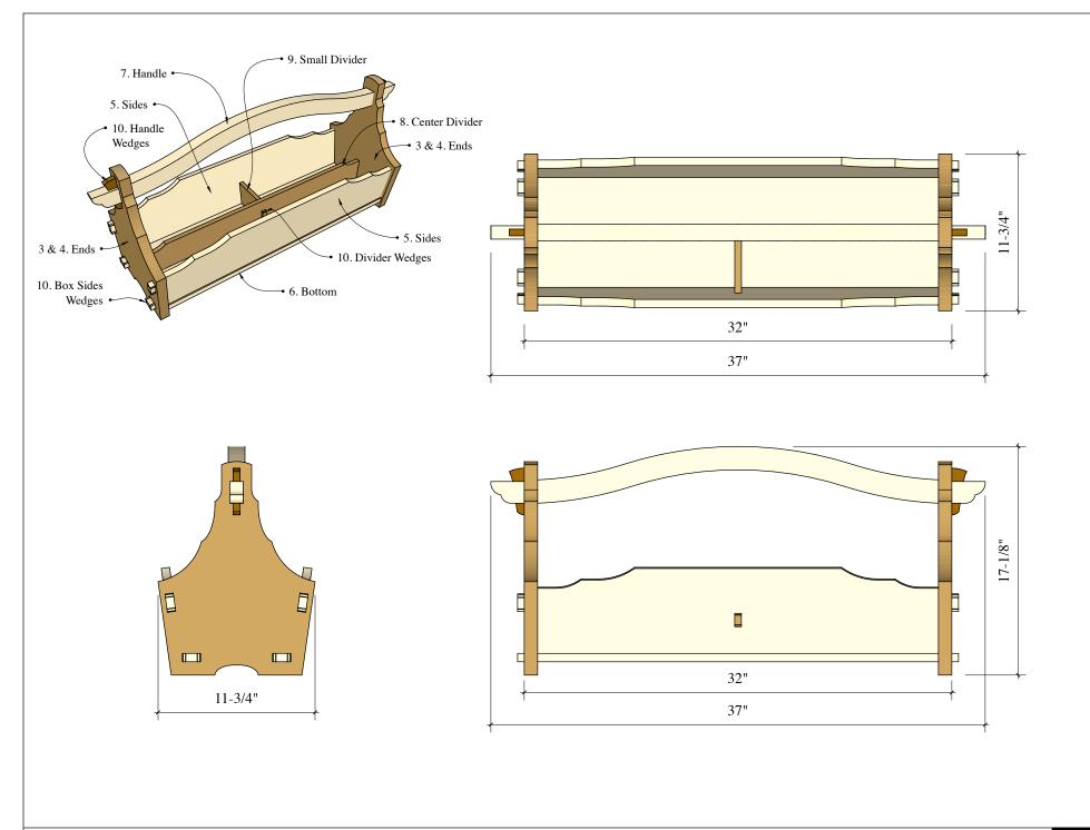
IRAI Toolbox NTER www.samuraicarpenter.com NOTE: The dimensions listed below are finished dimensions and extra length and thickness should be added when calculating the material needed.
