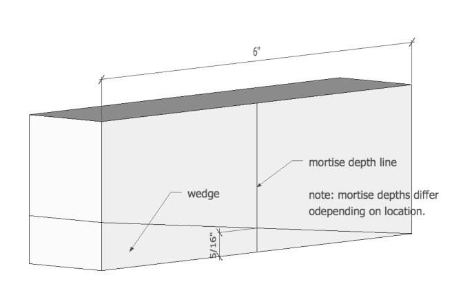
note: cut wedges 2" longer then the tenon and taper from 0" to 5/16" over the depth of the mortise. example above.
